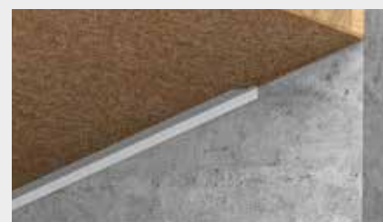
Sealing a wood floor connecting to a plastered wall
