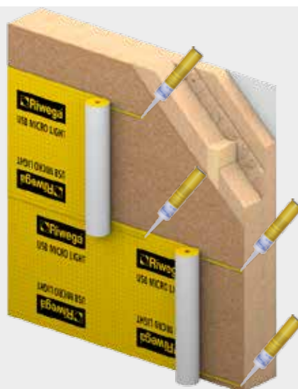
Gluing of USB Riwega vapour control layers/barriers on internal wooden walls or OSB boards with sealing of overlaps
