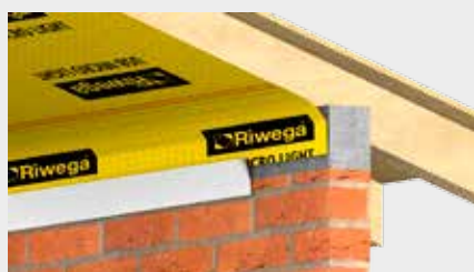
Sealing a vapour control barrier applied to the interior of a roof when connecting to a plastered wall
